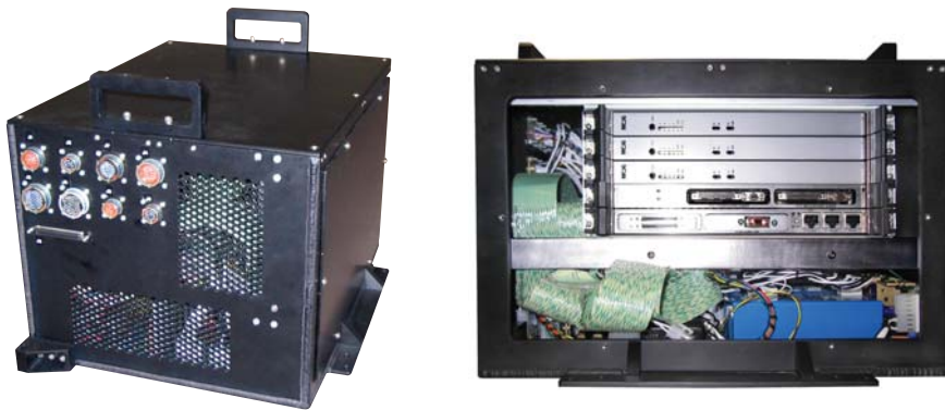
Figure 3. SCC's Integrated Sensor Data Processor (ISDP), slated for deployment in the Predator.
